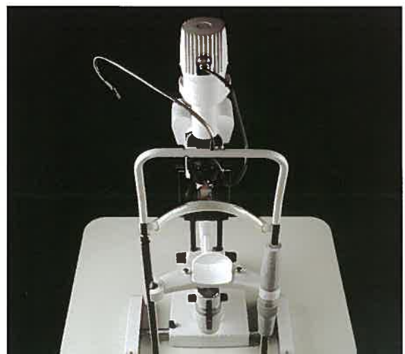
mod. MM 5 Galilean microscope 5 magnifications 6x - 10x - 16x - 25x - 40x
