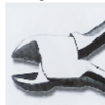
015 : Side Cutting Pliers to cut screws, lenses and general adjustments. Small or big size
